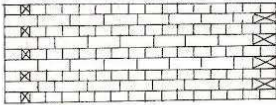
Elevation of wall in English cross-bond.
